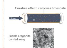
The AQUA4D® technology has an effect on the crystalline structure of the CaCO3 limescale, which changes to a friable, non-agglomerating state, aragonite, and the limescale no longer adheres to the surfaces.
